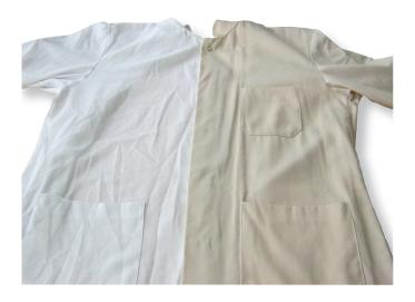
The textile on the left has been treated with Turbo super wetting before washing using a standard white workwear process. The textile on the right has not.
